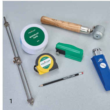
1 Standard installation tools. Only Polyflor QuickLay recommended double-sided tape should be used.
